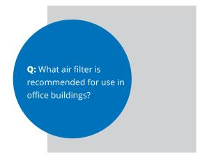
A: ASHRAE recommends MERV-13 filters or higher. When systems cannot handle the increased size or air pressure, an electrostatically treated filter can be used to meet the MERV-13 rating.
